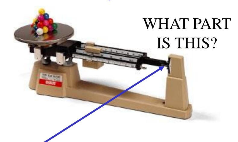
This is the pointer: It points to ZERO when the balance is correct.
